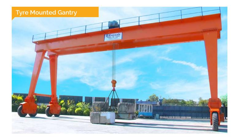
Amsak Rubber tyre gantry cranes (RTGs) delivers exceptional productivity and reliability in Coil / Container stacking. They are available with spans of between 20 mts to 30 Mts. They have a rigid and stable steel structure allowing precise handling with smooth movements even at high speeds. The high quality standard is achieved with ease of maintenance and results in minimum downtime increasing throughput per RTG Unit.
