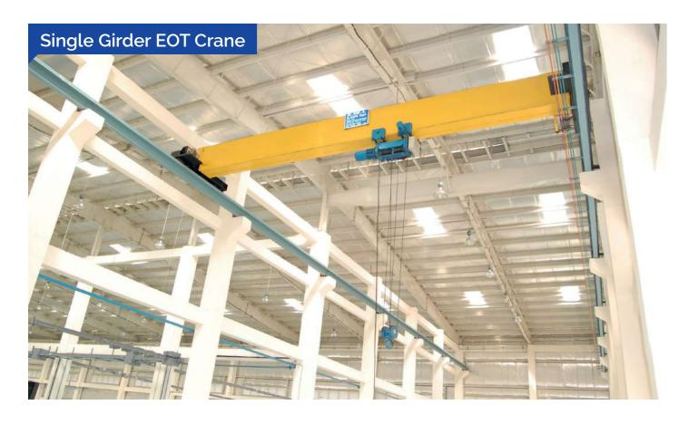
Single Girder Cranes are designed to cover a wide range of modern industrial demands, providing excellent value for money with no compromise on performance. Amsak's single girder crane has reduced wheel loads, saving costs on new support structures and increased lifting capacities on existing structures.
